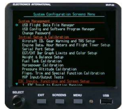
System Configuration Screens
